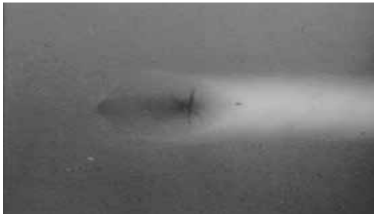
Figure 6-1: Radiograph Showing a Crater Crack
