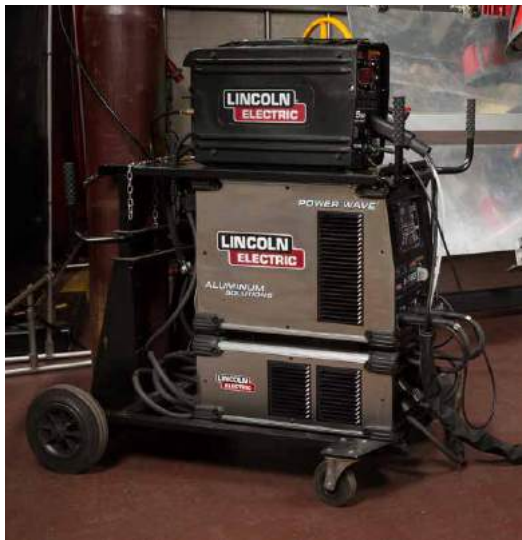
Figure 5-4a: Power Source with Advanced Module
